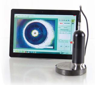
CCD camera system for Brinell hardness and indentation analysis. Have your Brinell hardness tests conducted and analysed with variable statistical functions offered by the Bullseye measurement analysis software. The digital analysis significantly reduces the uncertainty of measuring procedure and helps you to achieve quick and precise results as well.
